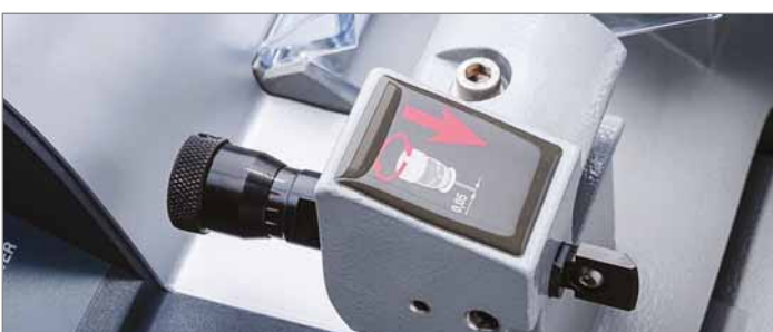
Bravo Evolution: micrometric tracer point
