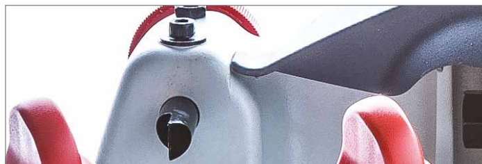
Tracer point with micrometric adjustment
