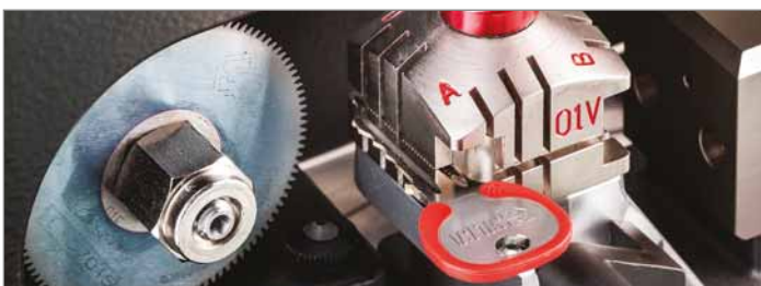
Flat and cruciform key cutting
